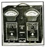
Test unit: wide-range scales—to 20 megs., 1,000 V. D.C., 800 V. A.C. 16 mf. and 500 ma. (1436)
